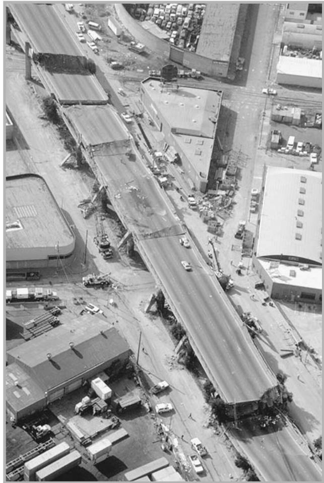
**Fig. 10.7** Aerial view of collapsed sections of the Cypress viaduct of Interstate Highway 880 (H.G. Wilshire, U.S. Geological Survey, <<http://wrgis.wr.usgs.gov/dds/dds-29/>>).
