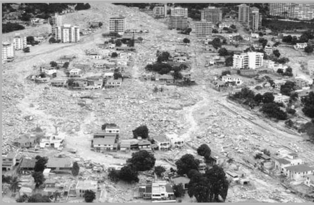
**Fig. 12.11** Aerial view of erosion and debris flow deposition during the Caracas, Venezuela, urban flood of December 1999. The deposit is up to 6 m in thickness and contains 1.9 million m<sup>3</sup> of sediment. Gaps denote areas where buildings were removed by the floods (photo by Lawson Smith, United States Geological Survey, <<http://pubs.usgs.gov/of/2001/ofr-01-0144/Venezuela/tnhires/pages/image030.htm>>).
